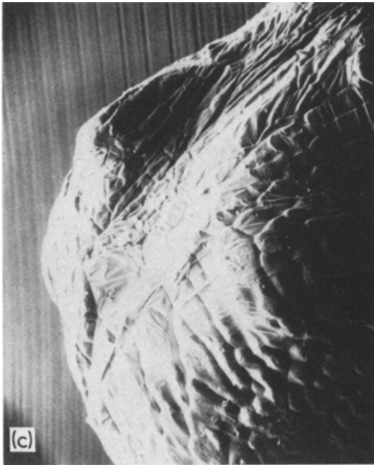
Figure 7 SEM views of atomized pure (99.99%) Al powders made utilizing an \text{Al}_2\text{O}_3 filter with average pore size of 87 to 100 \mu\text{m} . (a) \times 50 ; (b) and (c) \times 590 .
